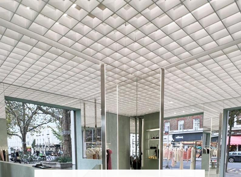
The unique ceiling design made us rethink how lighting can function within a space. As all lighting was above a bespoke made to measure ceiling raft it meant we had to install all electrical services prior to the raft being installed. All measurements had to be perfect in order to give the client the aesthetic look they required.
